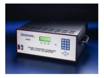
The internal photometer measures the actual amount of ozone generated, and corrects for errors, using closed-loop PID control. The photometer also allows an external source of ozone to be analyzed and displayed on the screen. The external ozone is connector to a separate sample port, allowing for simultaneous gas blending while monitoring the external ozone source.
